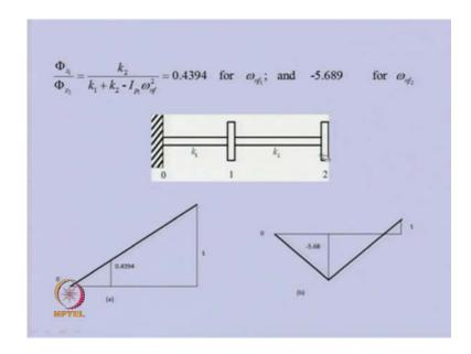
So, for first natural frequency, this is the value and for second is negative. So, you can able to see that we have more check corresponding to the first natural frequency. This is 0 station fixed, disc one location disc displacement, and here if you are taking unit displacement at station 2, the station 1 will be having 0.4394 unit on displacement. Similarly, here you can able to see that these two discs will be having anti phase motion for the second module.
