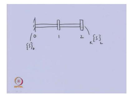
So, in this particular case we let us see, if we have two discs? So, this can be 0 station, this 1 station, 2 station. So, you can able to see that we need to relate the state vector, which is here right of 2 2 state vector right of or there is no disc. So, at 0 station once we
