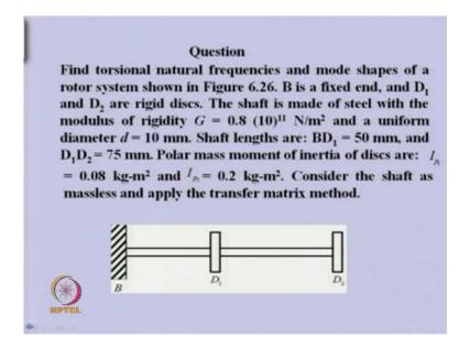
In this particular case the example is like this, so example is this one, we have a canteen liver beam in which two disc are there. Various property of the disc lens and everything is given here. We are considering the shaft as mass less only inertia are there at the disc. This end is fixed and other end of this is free.
