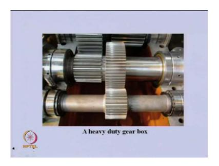
So, this is a typical application where we have a torsional oscillation there is the gear system in which we transmit lots of power and these gears gives a impulses in the form of talk. This may give torsional form torsional excitation in the form of vibration and any of the natural frequency in the torsional mode is coinciding with these gear mess frequency. Then we may have torsional oscillations in the resonance condition in the system similar to the gear system.
