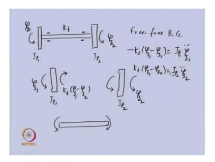
Now, let us take two disc system 2 disc that is connected by flexible mass less shaft this discs I p 1, I p 2 the shaft is having torsional stiffness k t, the shaft is having torsional stiffness k t and this shaft is supported, let us say on friction as bearing. So, that this disc I have angular displacement I am taking both as counter clockwise direction as positive, so this bearings are not provided as friction.
