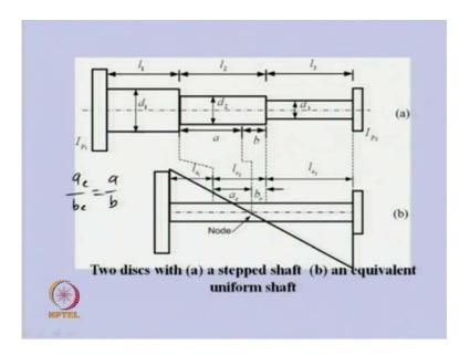
So, let us see what is the difference especially if we obtain the previous node position I in this particular case when we want the node position in the stepped shaft. So, this is the node position in the equivalent shaft corresponding to the second shaft segment. We will see that you can able to see that this dotted line is representing that from here to here is
