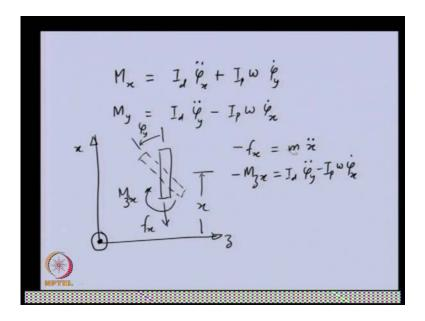
So, this will be I am drawing the free body diagram of the disc z x plane. So, this the disc this is the x displacement of the disc translator displacement, apart from this it is telting in positive y direction. That is f e y y axis is perpendicular to the screen and it is coming outside the screen. So, this particular point presenting the tip of the arrow of the y axis and because of this displacements we will be having f x in downward direction opposite to the displacement.
