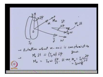
We are considering the disc like this. This particular disc is having this is the axis about which it is spinning the positive action direction, that is z axis. There are two ware axis in this particular disc x and y. This particular disc is having four moment inertia about z axis I p, because of this spinning the angular movement AM from the disc is let us say I p omega. In the positive z direction we restricted the rotation of this particular disc about x axis.
