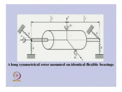
So, this is the rotor system which is supported on buy springs on two directions. Now, we have given the value of this particular case and especially we are interested in this particular case coupling between the translator motion and the. So, we could have able to analyze this in the translator motion tilting motion separately without any problem and based on our experience now we can able to write the equation of motion system like this.
