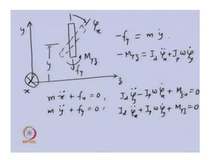
In z y plane for this let us consider the list having this y displacement and titling is in positive x direction. Then it is positive x, x axis is perpendicular to the screen and going into the screen cross is representing. That we are looking into the telt of the x which is inside the screen because of this displacement from the shaft will be having elastic force reaction force. Apart from that reaction movement from the shaft that will be y z.
