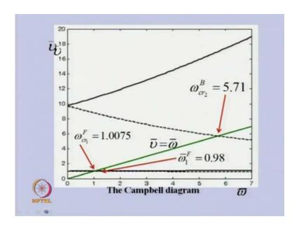
We will get a diagram like this is called Campbell diagram. So, horizontal axis is omega bar and what vertical axis is mu bar. So, you can able to see that we have this two lines, this splitting of the natural frequency is taking place, what is splitting is less for the first whirl. You can able to see this green line is nothing but mu is equal to omega line. There is a to critical split line, wherever this critical line is intersecting the frequency goes there, the critical speed.
