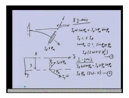
Now, we are able to get the angular momentum of the disc because this particular disc is tilting about its diameter. This diameter or so we need to consider the four angular momentum calculation for I d diameter mass momentum equation and will be
