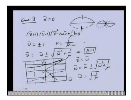
So, that means if we substitute this into this expression mu bar is equal to omega bar and we will solve for omega. Then we will get omega bar is equal to omega bar plus or minus omega bar square plus 1 mu. If we solve for omega we get the critical speed and this particular case we will see that one of the critical speed. If we solve this for omega will be minus 1 by mu.
