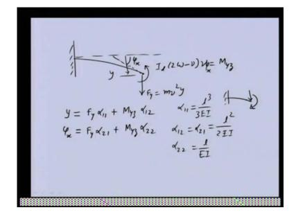
So, if we summarize we have now on to the shaft, if we remove the disc gyroscopic moment which we this the moment on to the shaft. So, this is opposite to what we got on to the disc. So, this will be outside the screen direction to this angular momentum and well U is I d 2 omega minus mu and this is mu we have seen earlier because of the linear motion that means displacement y. We had net resultant center figure force F y, it was acting downward this is the gyroscopic moment.
