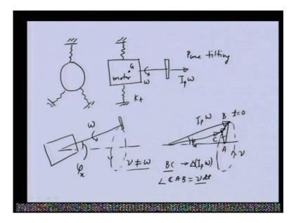
For this particular case; we will let us say there is a motor, and there is a rigid shaft, and there is a rigid disc attached to this. So, this whole assembly motor, the shaft and the disc
