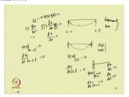
So, for example in case of this simply supported beam, the boundary conditions are so, in this at x equal to 0 and x equal to 1 boundary conditions are the both displacement and slope equal to 0 so, both displacement and slope equal to 0 here and in case of a no so, in case of the simply supported beam. So, here slope is not equal to 0 one can see that slope
