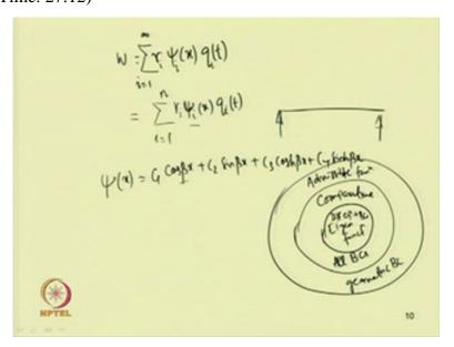
And time modulation and safe function so, one can write this W equal to r psi x into q t. Where, r is the scaling factor, psi is the safe function and q t is the time modulation. So,
