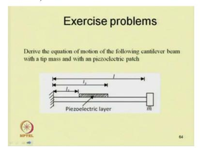
So, one can take this as one exercise problem and some other exercise problem also you can take to derive the equation motion. So, already you have seen this example so, also one can derive the equation motion for the sandwich beam when this magnetic field is applied one can find the equation motion by using the force due to magnetic field. Also one can derive the equation motion for a cantilever beam by taking piezoelectric layer.
