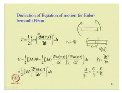
So, in case of the Euler Bernoulli beam, the beam is subjected to pure moment pure bending moment. So, in this case as the beam is subjected to pure bending one can derive the equation motion for the system by taking the kinetic energy and potential energy of the system.
