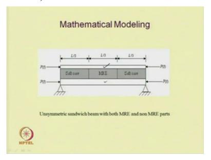
And you can take some exercise problems also where you can derive the equation motion for a sandwich beam so, in the sandwich beam 3 so, this is the core element both are both are skin and this is core so, in this core one can use this Visco-elastic or elastic material also one can use this magnetorheological elastomer also, by taking different property and taking this force so, one can derive the equation motion.
