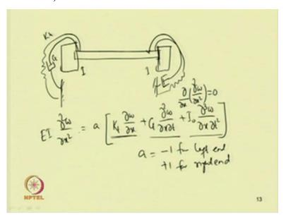
By taking a torsional spring and damper in this case one can have let us take a rotary mass also, a mass with moment of inertia I and let us take a torsional spring and torsional damper. So, in case of this torsional spring that of this is a torsional spring and let us take a damper this way similarly, this side also one can take a spring and damper and let I is the moment of inertia then, this is the damping element and one can have a spring element also torsional spring element.
