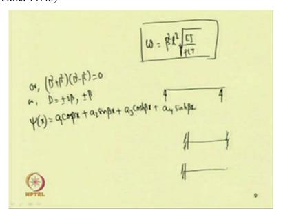
The auxiliary equation becomes d forth minus beta forth equal to 0 or d square plus beta square into d square minus beta square equal to 0 or d will be equal to plus minus i beta and so, this will give so, it will be or it will be plus minus beta so, one can 4 root and from this 4 roots one can find the general solution for psi x. So, general solution for psi x
