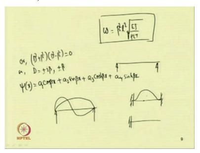
So, for example in case of the simply supported case so, one can obtain the first mode like this so, displacement will be 0 at both the ends. So, similarly, for the second mode so, there will be node formation here so, the displacement will be like this and similarly, for second node second mode there will be 2 nodes and incase of a and incase of fixed fix the first mode will be so there will be slope and displacement 0 at both the ends so, it
