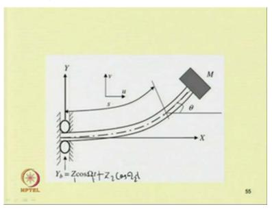
Base excited cantilever beam where the base motion can be given by z 1 cos omega t and z 2 cos omega 2 t. So, in this case it will be subjected to 2 frequency excitation you can take multi frequency excitation also.
