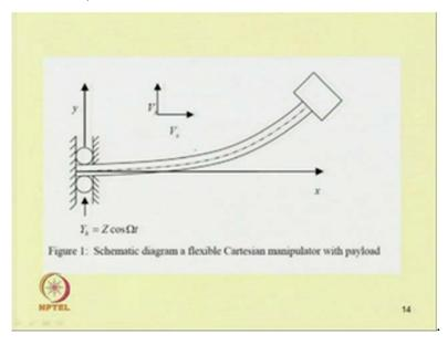
So, in this case so, let us take this example so which so a Cartesian manipulator with a payload or which can be modeled as a cantilevered beam where, the left end is roller supported and which can move up and down and let us consider the large transverse vibration of the beam. So, as we have seen before so, in case of the large vibration so, this M can be written instead of writing M equal to E I del square y by del x square, one can write that equation in this form.
