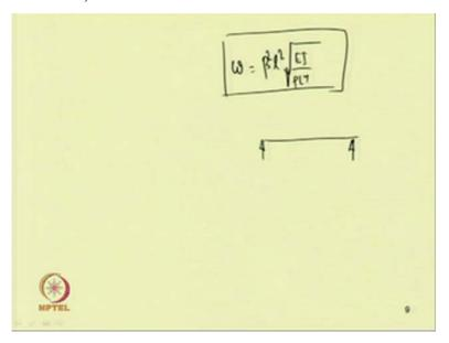
Or if one multiply 1 so, this omega can be written as so, omega can be written as beta square 1 square root over E I by rho 1 forth and one can so, from this equation one can find the expression for psi that is the safe function for different boundary conditions. For example, let us take the simply supported case.
