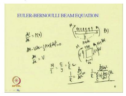
So, if one takes large deflection so, in that case this 1 by R will be replaced by del square y by del x square by 1 plus del y by del x whole square to the power 3 by 2.
