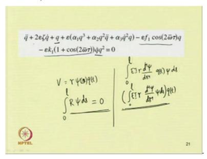
So, one can apply the galerkin method and one can reduce this equation to that of the temporal form where the equation in space and time is written only in terms of the time coordinate that is q or time modulation and the space part becomes the coefficient of that term. So, by taking a known safe function or by taking the known Eigen function of the system so, one can easily find these coefficients and one can convert these equations in
