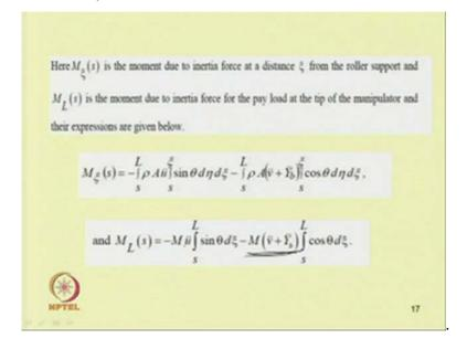
So this will be equal to minus M u double dot integration s 2 L sin theta d zeta minus M. So, this is due to the axial this is due the vertical direction inertia force and this is due to the axial direction inertia force.
