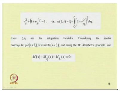
So, taking those inertia forces so, we can find the moment or we can find we can so, at a distance zeta so, one can write this one can find this bending moment also.
