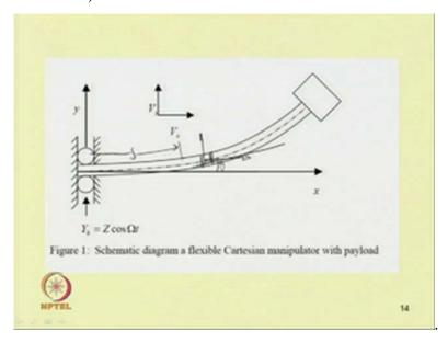
So, where theta is the angle between so, this is this angle is theta. So, when taking the moment so, one can take the moment about this point so, one can have this cos component and sin component. So, for axial and for vertical between one takes the moment so, then it can be written in this form. Similarly, this M L s that is due to the tip load so, one can write this equation M L s will be equal to this is the bending moment due to the tip load.
