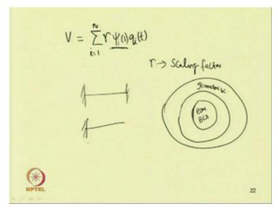
For example, in case of this fixed fix beam so, we have both geometric boundary conditions as at both ends the displacements and slopes which are geometric term are 0. But, in case of this cantilever beam the left end we have this geometric boundary condition but, in the right end we have the force boundary condition. So, in case of right end we have this sear force and bending moment equal to 0.
