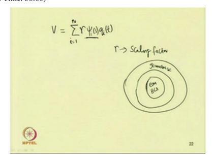
So, instead so, as a continuous system has infinite degrees of freedom so, instead of considering all the degrees of freedom one can truncate or one can consider only few modes for this analysis purpose. So one can limit this n to few modes and then perform this analysis. So, by taking this n let for example, taking n equal to 1, one can take the single mode approximation.
