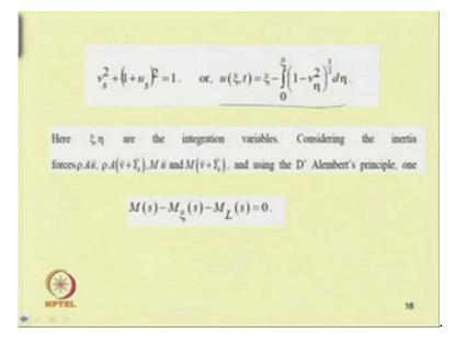
So, one can achieve this relation where del square del v by del s whole square plus 1 plus del u by del s whole square equal to 1. That means, the length remain constant if you are considering the length to be constant then one can have this in extensibility condition. Or in other word one can write this longitudinal displacement in terms of the transverse displacement using this relation.
