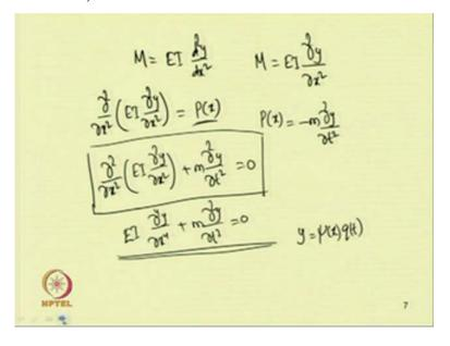
And one can expand this term by taking thing to numerator and have a non-linear equation. So, let us first solve this linear equation or let us see what the importance of this equation is or how it can be solved. So, one can take the variable separation method by considering y equal to let one consider this y equal to psi x into q t so, where psi x is the safe function and q t is the time modulation.
