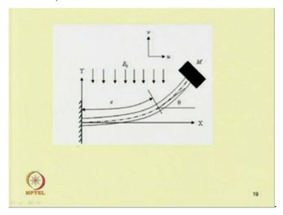
And couple in addition to the inertia force acting at a distance s from the base of the beam. So, by taking all those forces into account and by applying this d'Alembert principle one can obtain the equation motion.
