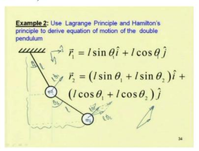
And then for the second mass or one can directly also write the velocity of these so, velocity of this is nothing but, this is equal to 1 theta 1 dot so, the velocity of this point equal to 1 theta 1 dot and velocity of this point will be velocity of this, of the first one parallel to this one can draw a line parallel to the first one plus the velocity of this point with respect velocity of this point with respect to this so, which perpendicular to this link.
