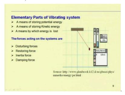
So, in the last class we have seen for these vibrating systems, this is the simple pendulum in which this kinetic energy is converted to potential energy and vice versa. So, the total energy of the system remains constant. So, by using this energy based principle also, we have to derive this equation motion.
