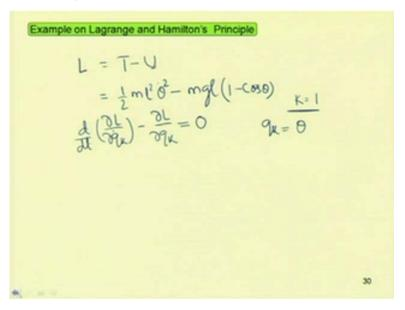
So, already you have found the potential energy this is m g l into 1 minus cos theta. Now, has to use this Lagrange principle and then Hamilton principle to derive this equation of motion. So, using Lagrange principle our equation motion can be obtained in this way so, d by d t of del L by del q k dot minus del L by del q k so, as no external force is acting on the system so, this will be equal to 0 and in this case q k that is the generalize coordinates so, k equal to 1.
