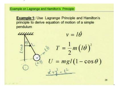
So, this is single degree of freedom system. So, k equal to 1 and q k is nothing but theta. So, one can take different coordinate systems also one can take x and y coordinate system but, if one takes x and y coordinate system to locate this position of this pendulum that time the equation can be retained in terms of x or y as x and y are related by this constant equation. That is, if this coordinate is x y then one can write x square plus y square equal to 1 square.
