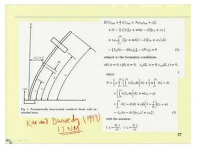
So, one you can refer the paper by Kar and Dwivedy 1999. So, this paper is from International Journal of Non-linear mechanics. So, the equation motion can be derived using this d'Alembert principle, by taking a small element, by writing the bending moment at this point one can derive the equation motion. So, in this way you can derive the equation motion. So, in the next class, we will use the Lagrange principle and extended Hamilton principle to derive the equation motion of different systems.
