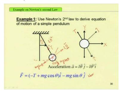
So, let us take or let us use this Newton's second law to derive the equation motion of this simple pendulum. So, in case of a simple pendulum this is bob with a massless rod. So, let me write this is my coordinate frame x y I can use a coordinate frame x y or I can use another coordinate frame also. So, I can take a unit vector along this direction that is and along this direction.
