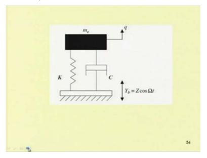
So, one can model the system like a spring mass damper system with moving base and find the equation motion also. So, let us see some quiz problem.
