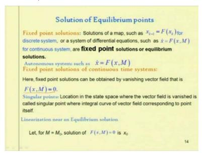
So, for these cases already we have discussed about the fix point by substituting this x dot equal to 0. So, we can write the fix point equal to F x m equal to 0. So, here m is the control parameter so either by linearization near the equilibrium position or by perturbing we can find or we can study the stability of the system.
