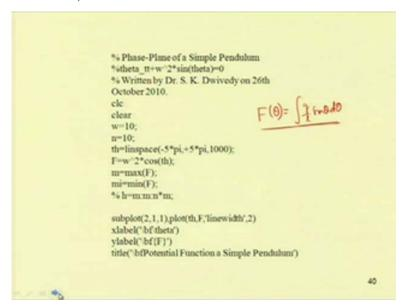
So, one can, one can write a program, simple matlab program to find the potential function. So, potential function F theta will be equal to. So, in this case F theta equal to g by 1 sin theta so, capital F theta will be. So, this will be equal to g by 1 sin theta b theta. So, this is 0 to 1. So, one can find this F theta. So, this will be g by 1 minus g by 1 cos theta. So, in this case it is written so, F equal to omega square cos theta.
