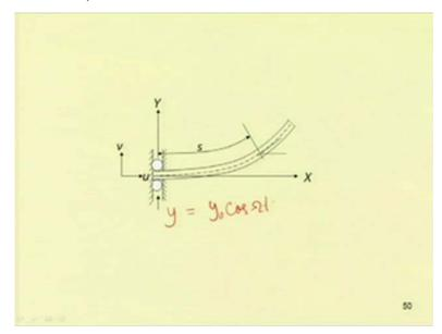
So, one can easily find the equation motion by using those scalar terms. Now, one more example we can see. So, in this case we have to derive the equation motion for cantilever beam, large cantilever beam which is subjected to a periodic force y equal to y 0 sin or cos omega t. So, let this y 0 cos omega t.
