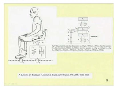
So, this is in the sitting position. So, the person is sitting on a chair so, if one can model this thing one can model the whole system by this spring and damper system. So, the leg part is modeled as true body to rigid body with the joints here. So, by taking all the spring and damper, spring mass damper one can develop a lumped parameter model for
