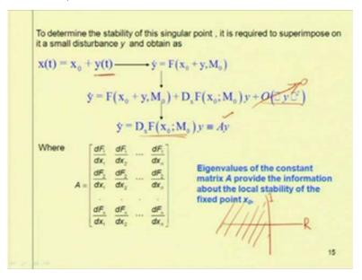
So, by taking a small parameter near the equilibrium position x 0 one can write the governing equation y dot equal to F x 0 plus y controlling parameter M 0. And by expanding this thing using Taylor series one can write this y dot equal to F x 0 plus y M
