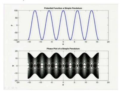
So, one can similarly find the theta dot term and if one plots so, this is the potential function and the resulting phase plot for the simple pendulum. So, these are the center
