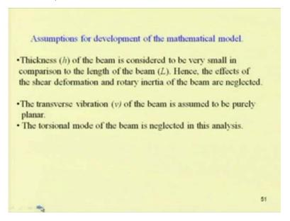
So, in this case one can take these assumptions, you can assume this as an Euler Bernoulli beam and derive the equation motion. So, by using Newton's second law one can write the bending movement equals to e i.
