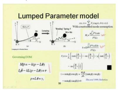
So, you can model the bending of the system like a bending spring and this mass you can take this mass of the mass of this part empty plus mass elastic mass. So, it can be taken
