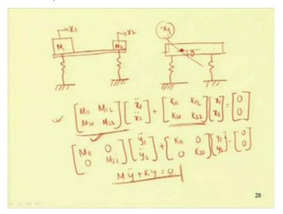
So, for example, in case of a leg machine, the leg machine can be modeled as a. So, this side one can model this as a spring and mass damper model spring and mass model. So, this is the mass of the head stuck m 1 and this is the mass of the tail stuck side. So, this is tail stuck side and this is head stuck side and this is the lathe bed. So, we are considering the mass to or the bed to be 0 or one can model this as a mass a centrically placed mass also. So, the mass can be put at this position.
