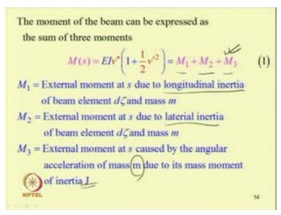
So differentiating it twice, so, you can write this u double dot in this way. So now introducing this we can write the governing equation motion using Hamilton or using this differentiating this equation twice. Now substituting this expression for M1 M 2 M 3 in this equation and differentiating this equation twice as we are differentiating.
