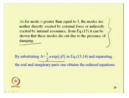
So we can write this equation in this way, so these are known as the reduced equation. So in this case we are getting four equations, so these four equations are known as the reduced equation. So this equation so these equations can be written so this is the first equation, 2 omega 1 zeta 1 A 1 plus A 1 dash minus half f 1 1, so this is the forcing term f 1 1 A 1 sin 2 gamma 1 so here we have initially we have substitute A equal to half A E to the power i beta.
