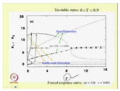
So this is the so here also one can see several bifurcation points and here one may note that after this point as there is no stable state present in the system, the system will fail due to this catastrophic blue sky catastrophe phenomena and here one can explain the jump up and jump down phenomena in the system, for example, by increasing this gamma from this position one can see the system will rest jump from point to this point.
