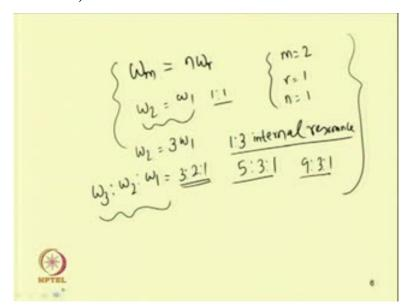
So already we know a system is said to be internally resonance when frequencies, that is the model frequencies let the model frequencies omega m, if omega m can be written as n omega r. So where m and r are the model frequencies for example, m equal to 2, r equal to 1 and let me take n equal to 1. So in this case omega 2 equal to omega 1, so this is known as 1 is to 1 internal resonance. Similarly if omega 2 equal to 3 times omega 1, so this is known as 1 is to 3 internal resonance.
