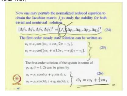
Now one can easily perturb this equation to find the response or stability of the system. So now by perturbing this equation one can write or one can find the Jacobian matrix, so Jacobian matrix j c, so which is the which is obtained by the first derivative of the terms of that equation. So one can write or one can find the Jacobian matrix, so after finding this Jacobian matrix so one can find the solution.
