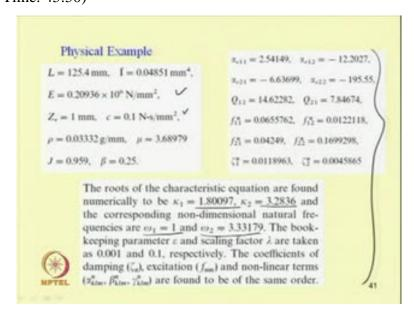
So solve the reduced equation reduced order equation numerically to obtain the steady state response, so use the obtained response as initial condition in the Newton's method for solving the set of non-linear equations obtained by substituting the time derivative terms equal to 0. So generate more and more initial points to use it in the Newton's method for different frequency conditions.
