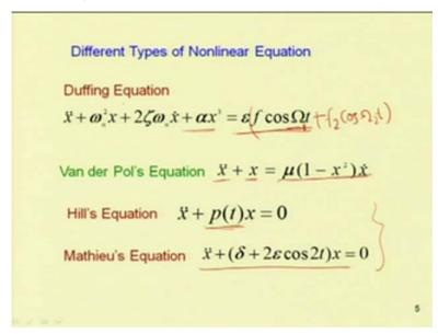
So, last class we have seen four different types of equations: one is Duffing equation, which can be commonly derived from a spring mass damper system with by taking a spring mass damper system with non-linear damp non-linear spring.
