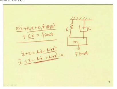
So, let us take the system. So, this is a spring mass damper system, this is mass m, spring constant k, this is c. So, if the spring constant, if the spring is not linear spring or it is a non-linear spring then, the equation motion for this system can be written in this form.
