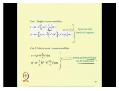
So, in that case, in that case, one will get this; one will get this reduced equation. Now, in this reduced equation by substituting this a dot and gamma dot equal to 0 for the steady
