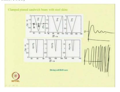
For example, let us take this instability region here. So, here if one take a point here here and here. So, this point corresponding to A. So, if one plot the time response. So, it will lead to a stable condition. So, it will finally, lead to stable condition which is 0 trivial state similarly for this C also it will lead to trivial state and for one can take B then the
