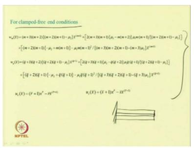
So, this is for clamped free end condition. So, in case of clamped free end condition. So, this is clamped and this is free or this is a cantilever type. So, in this cantilever sandwich beam this is a cantilever sandwich beam.
