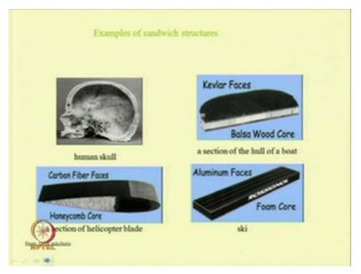
So, example of the some of the sandwich beams. So, human skull is the natural sandwich beam and. So, these are the carbon fiber faces one can use this honeycomb core. So, this is section of the helicopter blade where one can use this sandwich beam similarly this is a balsa wood core kevlar face also this is foam face with aluminum. So, foam core aluminum face and one can use this magnetorheological elastomer also.
