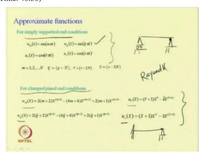
So, here we can take this w m w q u r and u s as the safe functions of the corresponding Euler Bernoulli beam with boundary condition. So, for example, in case of simply supported end condition. So, we can take this w m x bar equal sin m pi x bar similarly w q k bar these are the transverse direction thing. So, w q x bar equal to sin q bar pi x bar
