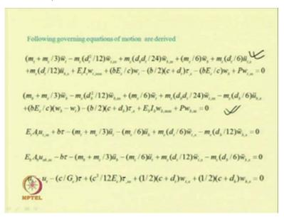
So, the coefficient of delta w t d x d t will be first equation similarly the coefficient of delta w b into d x d t will be the second equation similarly the term with u t and u b are u t double dot and u b double dot will be the other terms.
