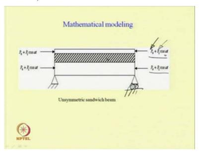
So, let us see the mathematical modeling of this sandwich beam. So, here a force P 0 cos omega t is applied. So, let us take unsymmetric sandwich beam with simply supported at the ends. So, it is subjected to axial force of P 0 plus P 1 cos omega t. So, P 0 is the static force and P 1 is the amplitude of the dynamic force with frequency omega. So, this is the
