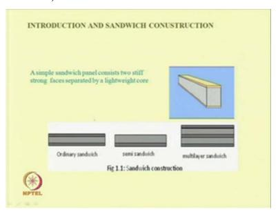
So, a sandwich beam. So, it can be of a ordinary sandwich beam or it is a semi sandwich where will have one singles skin and this is the viscoelastic layer. So, one can have multi layer sandwich beam also the sandwich beam may contain foam type of.
