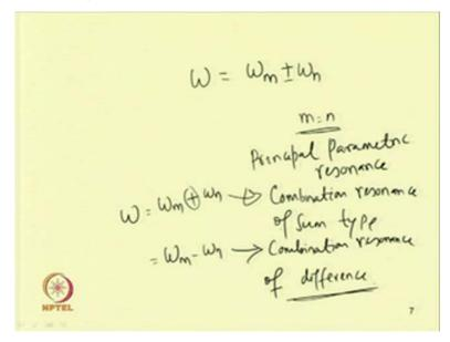
So, this parametric excitation will takes place at a frequency omega. So, so this will be equal to omega m plus minus omega n of the system. So, when m equal to n. So, this is known as principle parametric resonance principal parametric resonance condition and when m not equal to n then will have two conditions. So, one will be omega m plus omega n. So, where m.
