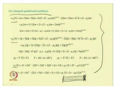
So, in that case we can have either we can have a guided this way or we can or we may. So, the guided condition we can have. So, it can be. So, it is constrain to move in this guide as we are considering the transverse vibration. So, it is constrain. So, this sandwich beam is constraint to move in this direction. So, we have roller support. So, this is for the clamped guided end condition. So, for the clamped guided end conditions you can use this w m w q and u s u r u s.
