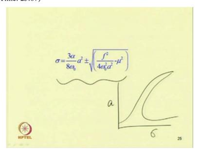
The response steady state response will be stable if the real part of the Eigen value becomes negative and it is unstable if the real part of the Eigen value is positive. So, one can plot.
