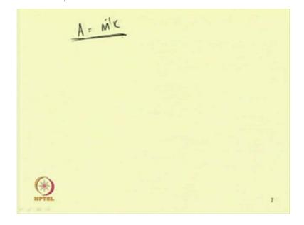
A let us find dynamic matrix A equal to M inverse k. So, if you write A equal to M inverse k and find the Eigen value of this. So, if we find the Eigen value of this and Eigen vector of this then we can write the model matrix.
