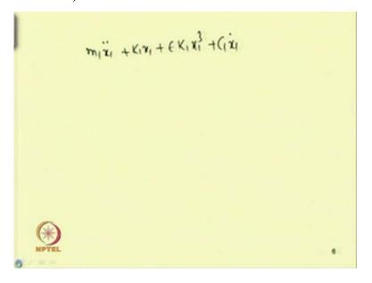
That means, m 1 x 1 double dot m 1 x 1 double dot plus f 1. So, for f 1 I can write this equation in this form that is k 1 x 1 plus epsilon k 1 x 1 cube. So, this is f 1 then plus c 1 x 1 dot c 1 x 1 dot. So, if I am applying a force.
