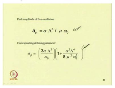
The free vibration amplitude of the system equal to alpha lambda mu cube by omega mu omega 0 and the corresponding detuning parameter is this. So, this is the super harmonic resonance condition and one can also study this sub harmonic resonance condition in. So, from this equation already we have seen the condition 3 omega equal to, So, 3 omega equal to by substituting 3 omega equal to omega 0.
