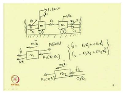
Let me apply a force capital F 1 F 1 sin omega t. So, that force, this will be equal to F 1 sin omega 1 t. So, I can write this equation.
