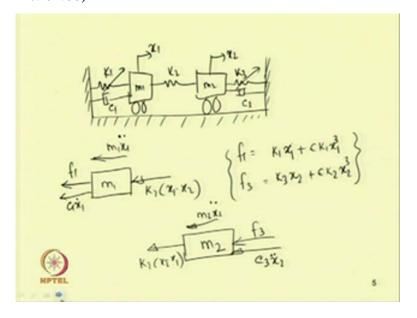
That is m 1 this case can be written in this form. So, this is subjected to a displacement x 1 towards right. So, it will be subjected to a inertia force of m 1 x 1 double dot towards
