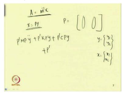
So, we can write the model matrix, in this case corresponding to these two. So, this is a two degree of freedom system. So, will have two Eigen values and corresponding to this two Eigen value will have two Eigen vectors. So, using this two Eigen vectors. So, we can uncoupled this equation by writing by using this thing P transpose M p p. So, by taking let us take this x equal to P Y.
