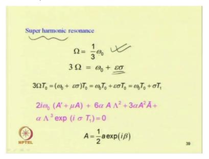
So, it will decay. So, we have the super harmonic resonance condition. So, we have seen the case 3 omega equal to omega 0. So, that is known as super harmonic resonance condition because in this case the system will oscillate at a frequency equal to omega which is equal to one third omega 0. So, this is super harmonic resonance condition. So, proceeding in the previous way, we can write this 3 omega equal to omega 0 plus epsilon
