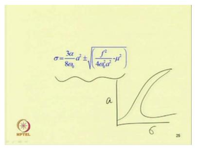
And this is the relation between the detuning parameter and response amplitude. So, by plotting the response amplitude verse detuning parameter, detuning parameter sigma. So, one can get. So, one can get the response like this. So, where it can observe the jump up or jump down phenomena and also one can study the stability of the system by finding the Eigen value of the equation these two reduced equation.
