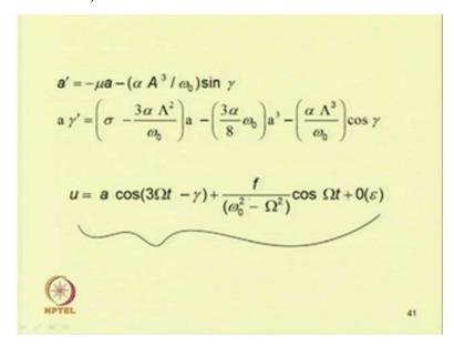
So, we have written this equation. So, this is the first order solution of the system. So, u equal to a cos 3 omega. So, this is a cos 3 omega t minus gamma plus f by omega 0 square minus omega square cos omega t plus order of epsilon.
