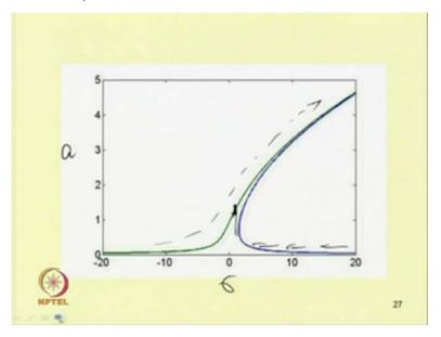
So, here by sweeping of so, one can. So, if it is super critical. So, one can follow this curve. So, it will go up, but while sweeping down the frequency. So, this is a versus sigma. So, by sweeping down the frequency one can observe. So, as here this branch is unstable. So, by sweeping down. So, one has as jump up phenomena here. So, it will the response will jump up and it will follow this curve again. So, one can have this jump up and jump up jump down phenomena.
