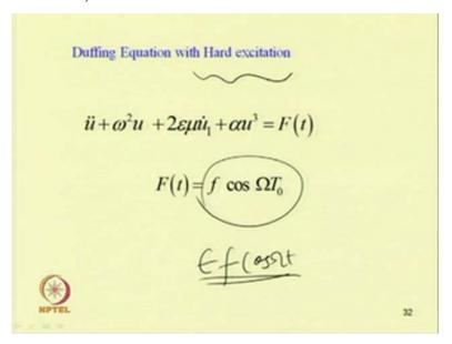
So, when the equation is hard excitation; that means, when we cannot write the forcing term as epsilon f cos omega t in the equation motion. So, here we are not using this epsilon. So, previous case we have written it is equal to epsilon f cos omega t, but in this as this terms no longer small.
