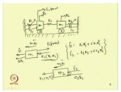
So, one can write this force. So, in the first equation I have to add this force k 2 into x 1 minus x 2.
