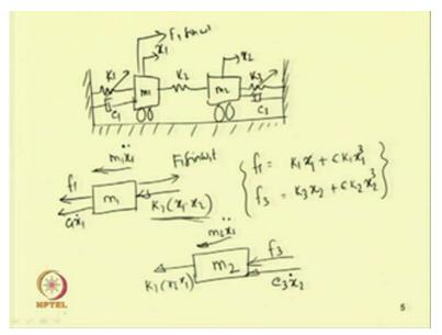
Let us see. So, what are the other forces acting. So, damping force plus c 3. So, damping force is x 2 dot not x 2 double dot c 3 x 2 dot.
