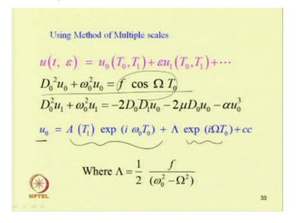
So, by proceeding in the similar way so, using method of multiple scale. So, we can see that the solution of this equation will contain two part previously as this right hand side was 0. So, we have only the complimentary part, but now in addition to this complimentary part we have to add the particular integral the system, particular integral
