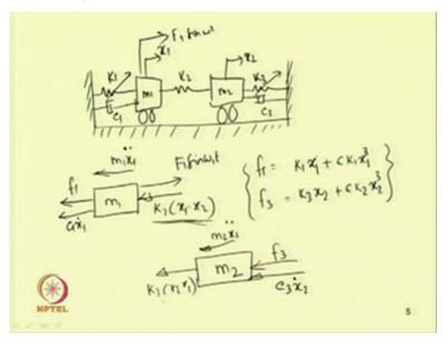
So, m 2 x 2 double dot. So, this is the force acting this way plus k 2 into x 2 minus x 1 k 2 into.
