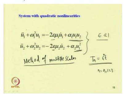
So let us take this non-linear systems with quadratic nonlinearity, so here we can write the equation two, we have taken a two degree of freedom system, where the equation is written u 1 double dot plus omega 1 square u 1 minus 2 epsilon mu 1 u 1 dot plus alpha 1 u 1 into u 2 then u 2 double dot equal to or u 2 double dot plus omega square u 2 equal to minus 2 epsilon mu 2 u 2 dot plus alpha 2 u 1 square.
