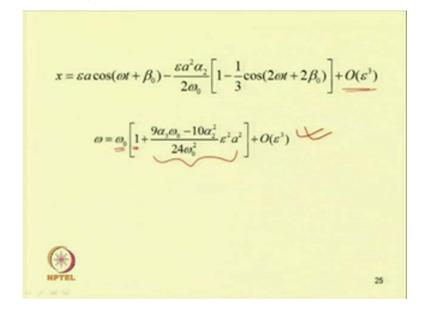
So, one can note that the resulting solution becomes so, as x equal to epsilon x 1 plus epsilon square x 2 taking only the first two terms so, we can write x equal to epsilon a cos omega d plus beta 0 minus epsilon a square alpha 2 by 2 omega 0 into 1 minus 1 by 3 cos 2 omega t plus 2 beta 0 plus order of epsilon cube.
