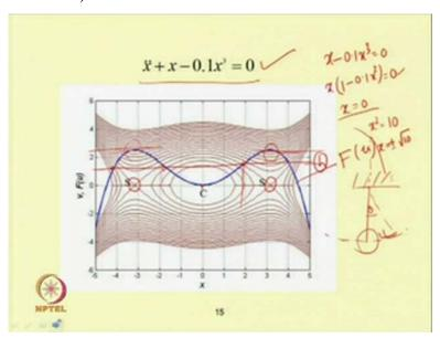
So, this is the line we have taken total h so, this is the h line so, this is the potential function. So, for this total energy h here so, we just see that these value up to this F u has a value less than h so, the motion will be so, we have corresponding to this value so, we have some motion and corresponding to this to this so, there will be no motion of the system and no so, as h is more than F u so, we have motion so, here F u is greater than h.
