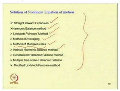
So, these are the different methods used for quantitative analysis so, in module two we made detailed discussions about how to find the solution of the non-linear equations by straight forward expansion method, harmonic balance method, Lindstedt poincare method method of averaging, method of multiple scales, intrinsic harmonic balance method generalized harmonic method, multiple time sale harmonic balance method and modified Lindstedt poincare methods.
