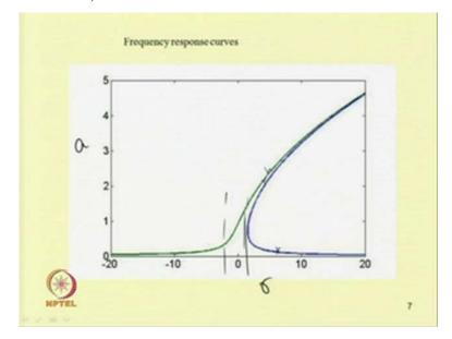
So we have only one solution, and for some other parameters so up to this, up to this, we have only single solution, and after that we have one, two, and three solutions. So after this value so we have three solutions, but or three branches. So here we have one, two, and three branch, and before that we have one branch of solution, so the question now arise, how to obtain this multi branch solution in this case of non-linear systems.
