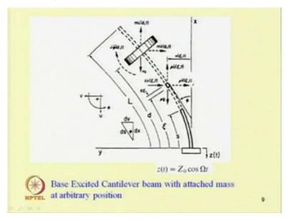
So let us take another example, so in this example, this is a base excited cantilever beam with attached mass at arbitrary position, so in this case for different position of the system, one can observe this internal resonance.
