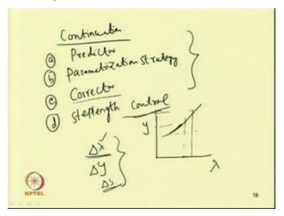
So our continuation method, so will contain a, so the continuation procedure what we are going to use, so it will have a predictor space, then which would have a parameterization strategy, how will parameterize that thing, so which would have this parameterization strategy, then we should have this corrector. And finally, we should find the step length,
