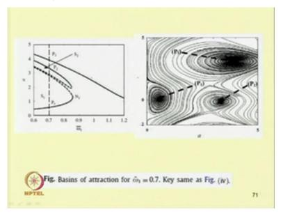
By taking different initial conditions, one can find the basin of attraction, when multiple solutions are present in the system. So, in this module, we have discussed about different numerical techniques for finding the time response, and the frequency response of the system. And in the next module, we will study about different applications of the non-linear methods, and the numerical techniques, what we have studied in this course.
