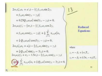
But in the present case the objective is to show, that in this case, if we are considering the internal resonance, so one can get a set of equations or one can by using this method of multiple scale. So, one can get a set of equation here considering 1 is to 3 internal resonance case, so here one can obtain four set of equations, so these are the four equations; unlike in case of this dufffing equation where one will get two reduced equations only.
