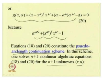
So from this or one can get this equation, so as we have this equal to 1 due to this condition, we have taken, so we have this equation, so equation 18 and 20, so this equation 18, so this equation and this x transpose t equal to 0, so they constitute this pseudo arc length continuation scheme, so in this scheme one solved n plus 1, non-linear algebraic equations 18 and 20, so for n plus one unknowns x an alpha, so after find that thing, then on each continue this scheme.
