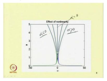
So, this is the frequency response curve. For this frequency response curve for this Duffing equation, or similar equation, equation similar to Duffing type, and so here the effect of nonlinearity is shown; so this is for alpha equal to 0, so these are for alpha less
