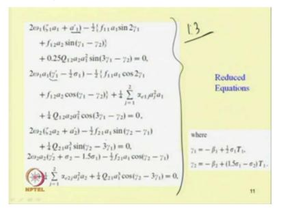
But, in the present case, so in this case, one has a set of four equations, so where this a 1 gamma 1 are for the first mod, and a 2 gamma 2 are for the second mod. So considering the two mod interaction, so where the first mod frequency is taken non dimensional, first mod frequency is taken to be 1, the second mod frequency is nearly 3 times the first mod; so here, 1 is to 3 internal resonance condition is considered, so in that case, so one can get a set of four equations.
