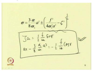
So, the reduced equation in case of Duffing equation can be written in this form, zeta a equal to 1 by 2 by omega n sin gamma, and this a gamma minus 3 by 8 alpha by omega n a cube equal to minus 1 by 2 f by omega 0 cos gamma; so this equations are written for the steady state, so one has two equations here, one can solve this two equation in case of the Duffing equation.
