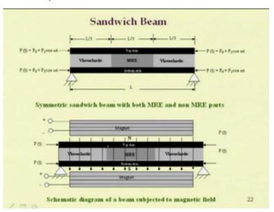
So, this is a sandwich beam. So, in case of the sandwich beam, you have a core and you have the skin and this core you can modify by taking different patches. So, you can add pejualact layer also, you may add magnetoriologicall Elastromer core also. So, in case of this magnetoriologicall elastromer core or can sort MRE for adding then, you can actively or passively you can control the vibration of the system.
