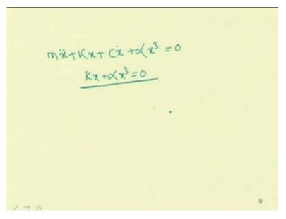
So, in this case for steady state I can have this k x plus alpha x cube equal to 0 and by solving this equation I can find the equilibrium position. So, one can make the qualitative analysis to study about the equilibrium position. How above the equilibrium position with time of the response behaves, that thing can be studied by using this qualitative analysis or quantitative analysis. So later, we will study about this qualitative and quantitative analysis.
