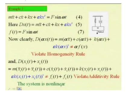
So, we have taken this example and we have studied these. For example, let us take the spring mass system. So, in this case of the spring mass system, if I will take a non-linear spring, then this equation motion can be written in this form that is m x double dot that is the inertia force, plus c x dot that is damping force and k is spring force.
