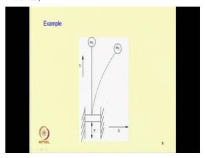
So, let us take the system, so in which, so we have a slender cantilever beam with one tip mass, and the base is excited and the base is moving up and down. Already, we know how to derive the equation motion of the system, the point of discussion in this case is, how we can numerically determine the system parameters. And then what other numerical techniques we are going to use in this case to solve or to find the response of
