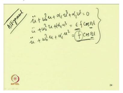
Duffing equation that is u double dot plus epsilon or u double dot plus omega 0 square u plus alpha 1 u cube plus alpha 2 u to the power 5 equal to 0. So, this is for free vibration of non-linearity and by taking so this left side equal to keeping this left side equal to constant as a or let me write it again. So, this is omega 0 square u plus alpha 1 u cube let us take the right side. So, this will be equal to epsilon f cos omega t, so this is the
