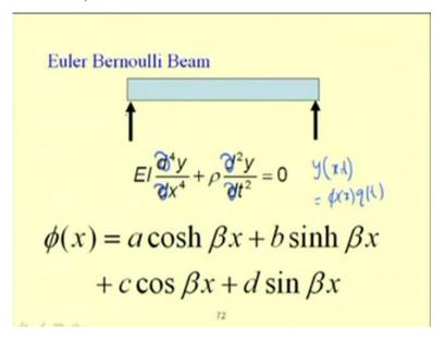
Similarly, for a beam beam in pure bending so in case of a beam in pure bending so one can use this Euler Bernoulli beam equation. So, in that case the equation can be written in this form e I del forth e I del forth. It will be replaced by partial differential equation del forth y by del x forth rho del square y by del t square equal to 0 because y is a function of both x and t.
