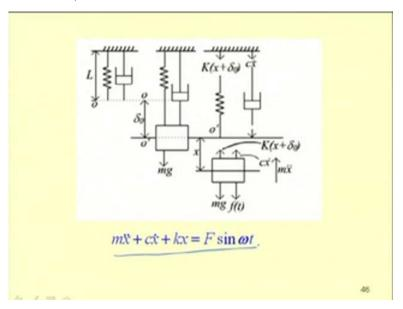
So, in this case so we have seen for example, for this spring mass damper system the equation of motion already, we know so that is m x double dot plus k x plus c x dot equal to f sine omega t.
