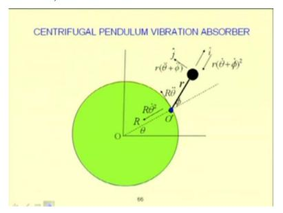
So, one may use this centrifugal type of pendulum vibration absorber for absorbing the vibration at different frequency. Similarly, one may use vibration damper to damp out the vibrations of the system.
