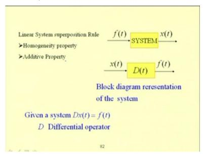
So, let us take a system so, the system incase of a linear system. If when we are applying a force f we are getting the response x so, in block diagram representation we can write x t equal to x t when applied here. So, this is d t and this is f t where d x t is the d is the differential operator.
