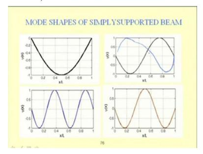
Like this and the mode shapes for a simply supported. For example, in case of simply supported the shape will be like this either it will be this or it may move upward or downward. So, this is downward it is shown one can have the upward motion also similarly, in this case one can have another motion also.
