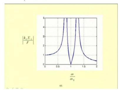
And left and it has a amplitude of 0 so this k one x 1 by f become 0 at omega equal to omega two, so when omega equal to omega two then this becomes zero.
