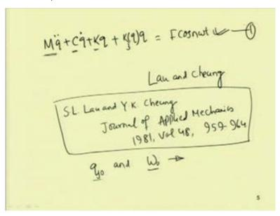
So, let us take the governing equation, general governing equation of motion in this form that is M q double dot plus C q dot plus K q. So, let us take a non-linear term which I can write in this form. So, this is a function of K 3 q. So, this is a function of non-linearity and then let me put a forcing term which I write in this form F cos n omega t.
