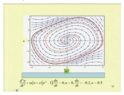
So, this is the flow. That is, the velocity u verses u dot curve. So, one can obtain this thing by solving directly the equation, Van der Pol equation. So, we show clearly a limit cycle solution and also one can plot this equation to find the same unit cycle.
