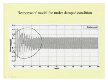
So, let us see this thing. So, for a under damped case so for a under damped case: one can see the initial part, which represent the transient part of the response, so it is varying with the initial condition, and it decreases, and finally it approaches a steady state response. So, this is the state response raised after several time steps. So, one can find the
