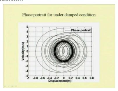
And, if one plot the phase portrait; so this phase portrait is plotted along with the transient part. That is why, it shows both transient and the steady state response part. This curve shows, the steady state part and starting for a initial condition. So, this shows the both transient and steady state part for this damped condition.
