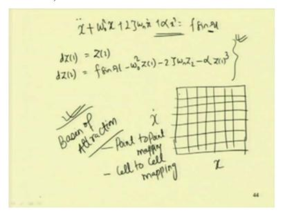
Let us take, the doffing equation. So, in case of the doffing equation; so x double dot plus, let us take a equation in this form: x double dot plus omega 0 square x plus 2 zeta omega n x dot plus alpha x cube, let it is equal to f sin omega t, so in this case, so one can write those two function; that is d z 1 equal to z 2, and the second equation d z 2.
