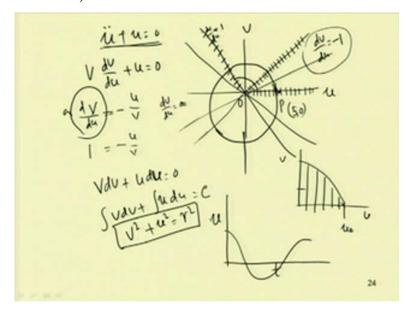
So, for example let us take the equation, u simple linear equation: u double dot plus u equal to 0. So in this case, one can write this equation in this form for u double dot. One can write this is equal to v into d u by v into d v by d u, so v into d v by d u plus u equal to 0 or one can write this v d v by d u equal to minus u by v, now by taking different value of d v by d.
