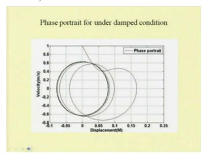
And, for the critically damped condition, so this response, this phase portrait represent the phase portrait for the critically damped case. And this represent for the under damped case.
