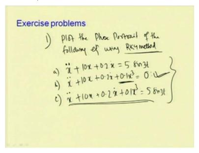
So, you can take few exercise problems to solve. So, plot the phase portrait of the equation, portrait of the following equation following equation; using RK4 method. So, in case of RK4 method, directly you can use the equations, what is shown, you can develop your own code or you can use mat lab to plot this thing. So, let you plot for this 1 x double dot plus 10 x plus 0.2 x dot equal to 5 sin 3 t, then x double dot plus 5 x plus 0.2 x dot plus 0.1 x cube, so this is duffing type.
