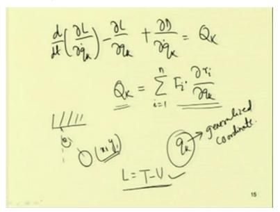
Similarly, in case of Lagrange principle so we can write the equation motion in this form that is d by d t of del L by del q k dot minus del L by del q k plus if damping is present in the system, we can write del D by del q k dot equal to q k so, where this q k that is the generalized force is written as summation i equal to 1 to n so F i dot del r i by del q k. So, here this let n number of forces are acting on the system then writing the position vector as r i.
