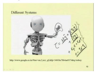
So similarly, in case of this humanoid robot to move this joint so for example, these fingers to manipulate these fingers so in that case one has to know, so what is the torque or force has to be applied by the tendant. So, there are several tendents in this humanoid robot, so in this humanoid robot also one can put the motor also at these joints, so one has to find what is the force or torque required at the joints in this robot.
