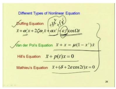
So, instead of using this Duffing equation, there are some more types of equation which we have also considered. This is Van der Pol type of equation x double dot plus x equal to mu into one minus x square into x dot, one can use a combination of this Duffing equation, and Van der Pol equation similarly, one can have this Hill's equation in this form, that is x double dot plus p t x equal to 0 and Mathieu equation in this form, that is x double dot plus delta plus 2 epsilon cos 2 t x equal to 0.
