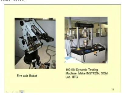
So, this is a five axis robot and this is u t m. So, in all these cases, one may observe that the parts are very rigid, due to this, to make it rigid or to make it very high stiffness one has to use heavy materials or make the components very heavy, but to reduce this weight for a different application for example, for space application to reduce the weight, one
