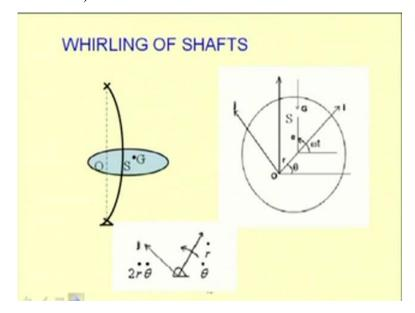
Similarly, one can study the whirling of a shaft, due to a bend shaft or due to the presence of one a centric mass in the disc, the system is subjected to a centrifugal force, so the plane containing the shaft access and the bearing line will rotate with increase in the speed of the shaft. So, that will cause whirling of the shaft, this whirling of the shaft is a transverse vibration of the system.
