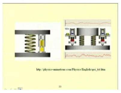
So, these slides show a spring and damper system, so this is the mass, during this vibration if it is very small or if the damping and the spring are assumed to be linear then one can see a linear motion or a simple harmonic motion.
