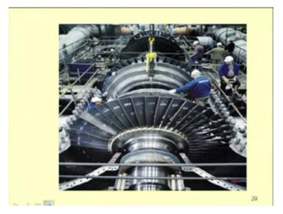
This is a turbine, these blades are shown, due to unbalance in this, sometimes unbalance may occur in this turbine blade, so due to that severe vibration may occur in this system. To avoid that vibration, nonlinear analysis may be required.
