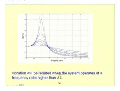
So this X by Y or F t by F 0, one can get same curve, one can isolate the vibration of the system, if it is operated at a frequency higher than root 2. And in that case one may observe, when it is operating at a speed greater than root 2 times the natural frequency, presence of damping will increase the amplitude of the motion. And before omega or if
