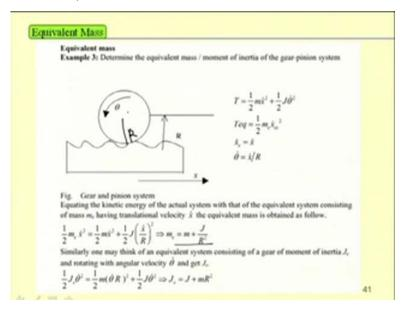
Similarly, taking this rack and pinion system, one can find the equivalent mass, one may convert this rack and pinion to an equivalent rotating system. In that case, at the speech point the velocity, is so if R is the radius of this pinion, then so R theta dot R theta dot, will be the velocity at the speech point for this pinion. And for the rack it is the x dot, it is the translational motion that is x dot, so at speech point the velocity is same.
