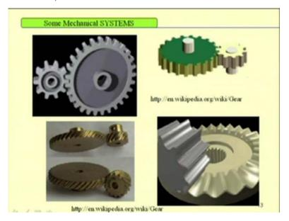
So, this page shows, so these are the some of the gears shown in these slides. This is a spur gear, so you can have spur gear, different types of gears, spur gear, vivel gears also you may have helical gears.
