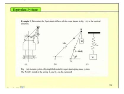
So, to find equivalent stiffness, for example, let us take this crane system. In this crane system, this rod and this beam, so one can find the equivalent spring for this one and finally, as it is moving in this direction, the mass is moving in the downward direction, so, one can find one equivalent stiffness of the system.
