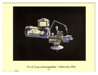
So, this is a long reach manipulator, this part in the long reach manipulator is used for repairing purpose in the satellite. In space crafts, due to weight constraint these long reach harms would be flexible, so due to the flexible nature they will be subjected to vibration. So, one cannot model this vibration to be small and in that case one will use the nonlinear vibration approach.
