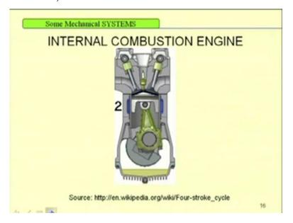
This slide shows the internal combustion engine, here also you can have several parts, so this is particularly a slider prank mechanism, in this slider prank mechanism one can have this unbalanced primary secondary or harmonic forces in the direction of line of stroke. Also you can have different parts, like the scum and other different parts which will be subjected to vibration due to this inherent unbalanced force present in the system.
