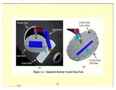
So, in this nuclear reactor, to open the nozzle valve one may use a robot, one may do this thing manually or one may use a robot, but due to this radioactive nature, a robot is preferable, but in that case also lot of vibration will occur if one considers a flexible manipulator.
