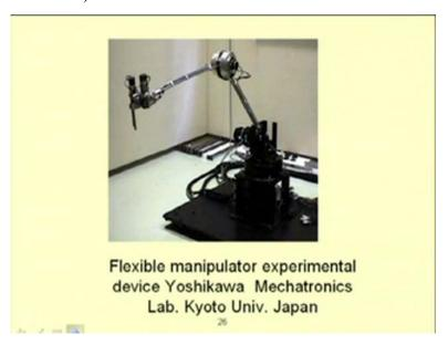
Here also a two link flexible manipulator is shown.
