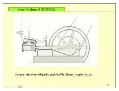
So, this is the animation for the steam engine, you can see different mechanical parts associated in the steam engine, you have a cylinder piston arrangement then this is the governor. The connecting rod, this is the crank, the crank is rotating this wheel. In this system, in this reciprocating system, one may observe inherent unbalanced force due to this inertia force associated in the system, also due to wear and tear in different mechanical parts one may observe severe vibrations.
