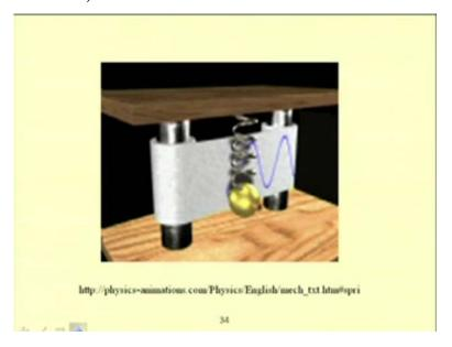
So, this slide, this animation shows a simple harmonic motion associated with a spring and mass system but, if the spring stiffness is not linear or if the spring is not linear so in that case the motion will be different type and in this course we are going to study what will be the motion if the spring is not a linear spring.
