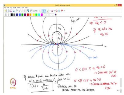
So, for u theta. So, if I look at theta between 0 and pi, which is the first two quadrants, in this case u theta which is given us minus mu by R square sine theta right, sine theta is positive in the first two quadrants, so, u theta would be negative which is what is defined in terms of
