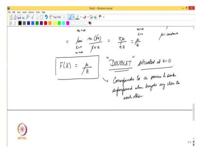
So, what we have reached is a complex potential F of z which is given by nu by z. This is a very important complex potential, which is what we call as a doublet. Doublet is made when you have a source and sink very near to each other. Now, this is also a doublet that is situated,
