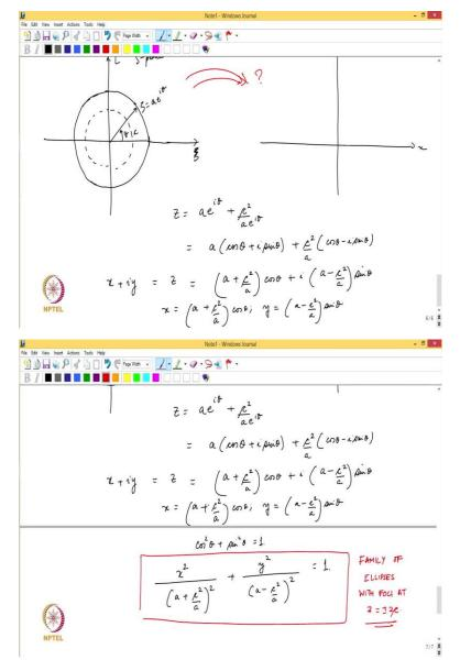
Now let us take another example with the same conformal mapping we still have z to be zeta plus c square by zeta, c is real. So, in the zeta plane we have zi in the eta coordinates. Now I want to look at how a new transformation works out in the jet plane which is given by the following. The transformation remains the same but except the representation I am going to use zeta is slightly different.
