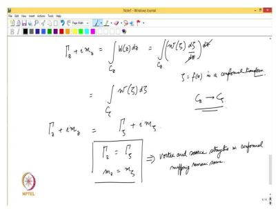
So, what we have come across now is that gamma let us say in the z plane plus Iota m in the z plane, subscript z denoting it is a z plane is integral W in the z plane dz integrated over a contour C in the z plane. I can write this integral by using the fact that W z which is the velocity in the z plane, it could be written in terms of velocity in the in the zeta plane. So, we could say this is for instance, w zeta times d zeta dz where zeta is f of z is a conformal transformation.
