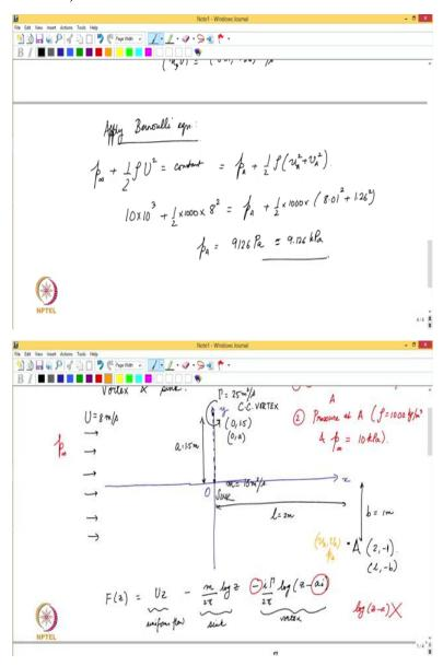
We can apply Bernoulli equation so we know that far away from the sink and the vortex pressure is p infinity and the velocity there is u, so we have p plus half rho u square to be constant in the flow ignoring all potential energy contributions. So, this should also be the same as p a plus half rho u a square plus v a square which is at point a, p a becomes a pressure at point a, u a b a are the components of velocity at point a.
