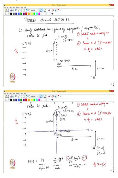
So, let us look at this problem which is about a 2D steady irrotational flow and this irrotational flow is formed by the superposition of say uniform flow, we have a vortex and then we have a sink and the vortex and the sink are placed at specific locations so say we have free stream uniform flow which has some velocity U the velocity is given say eight meter per second.
