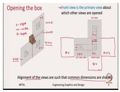
So, again we have this box and in that box we have this object, so we have captured the front view and after that we have capturing the top view. Now, comes the question, how do we unfold the box? So, the question here is we said that the front view is primary and we are not moving it, so which means the front view is fixed.
