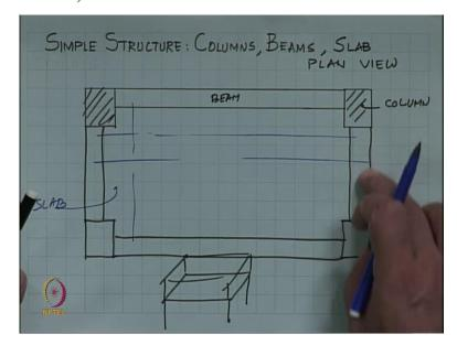
Besides the load-bearing wall, civil structures are of one more kind which is columns and beams. So, the difference is that we first erect a structure of beams and columns, then put the floors as a slab. So we can what we can add that here and then we erect the walls on these structures. So the walls that we now erect they do not carry the load.
