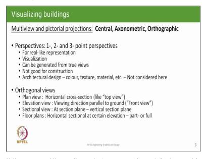
In visualizing buildings, we will use Central, Axonometric and Orthographic projections. But in this course, we will restrict ourselves to orthographic views. Perspectives, which could be 1-, 2-, 3- point perspectives, they are good for real like representation and visualization.
