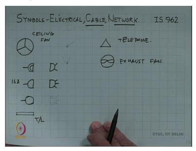
And finally, we come to symbols for electrical fittings. This one I have already shown is a ceiling fan. This is a plug for 5 A. This is a two-pin plug that is a plug for a power connection 16 A the three-pin socket would be like that and a light bracket on the wall would be like this during the plan view you showed this view on the wall if there is a light bracket there you need to have an electrical connection up to that point.
