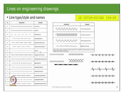
The line types that are used is very similar to the nomenclature that we had seen earlier. For instance, this has been taken from India standard 10714 which says that this type of line is called a continuous line, a dotted line, and if we go on down further, you have a double dotted line, you have dashed and dotted line, and so on.
