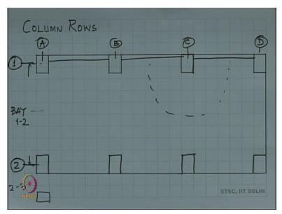
Another type of construction which is fairly large in size is a rows of columns. This is what you would see in a say a factory. So, what you have here is that you have this column here, this column here, this column here and with respect to the central line, we specify all their spacing and the column is specified by its dimensions which is this dimension and this dimension. So, all these columns and there could be hundreds of them one after the other all of that is classified as one row.
