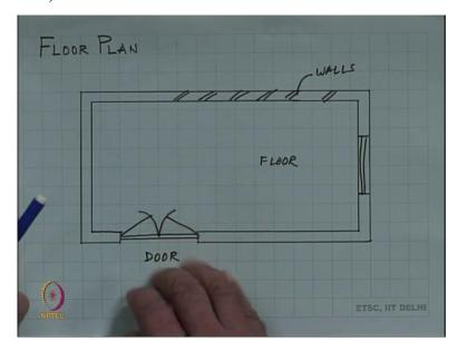
So, let us see how we can show these in orthogonal views. We will start by looking at what we call the floor plan, which means that if I cut this building. In a horizontal plane somewhere there all the way through, what will I see? So what we are looking at is typically a plane, which is cutting at some point here.
