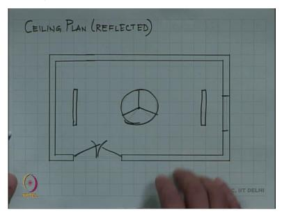
The other type of view is a ceiling view or the reflected plan which is what is it that we would see if we were to look up and say what is there on the ceiling. Now ceiling has several things on it. An example is a ceiling fan almost everybody has a ceiling fan.
