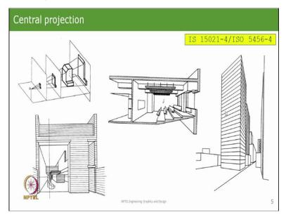
To revise what we had seen earlier in mechanical drawings, we had looked at Central projection, which is the way the human eye sees the surroundings. This picture on the top left is of a machine component. And it shows that depending on where the viewing plane is, we see the object in different sizes.
