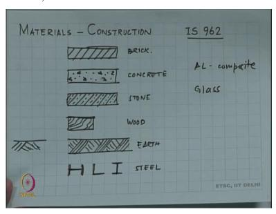
A quick note on various materials that are used in buildings and construction. The symbol with dashed lines there this design shown here it tells you that this is a brick construction. Then, if you have this symbol some large symbols like this and smart dots in between this is concrete.
