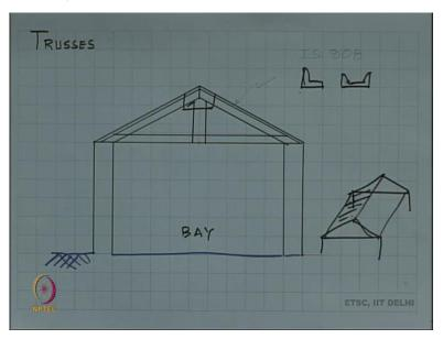
In industrial constructions. We put the columns as we have shown here. All of this is sitting on the ground inside this, this is the floor and outside this is the ground which is soil. On top of this these columns in one pair, we put a structure like this and this there could be lots of other designs on this. These are called trusses.
