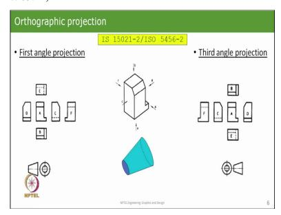
So, while these drawings are interesting, they do not meet the requirements that is there for design and construction which is where we go to true views which is orthographic projection, first angle projection, and third angle projection. In similar and architectural drawings, we follow largely similar ideas, but slight modifications.
