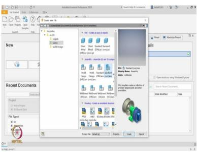
So here is the initial interface. Let us select the new template. So, we will select this metric system and we have a bunch of templates starting with the part model templates, assembly model templates, drawing and presentation templates. Since we are interested in the creating an assembly model. So let us go to these standard mm.iam, double clicking on it will take us to the assembly environment.
