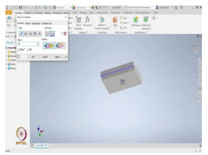
So let us get back to the constraint and now come back to the problem of how to bring these two blocks on top of each other. So, I will go use the constraint tool, I will use the first option which is mate. In mate it is asking for first selection.
