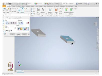
Now we will look into the second type of the constraint, which is the angle constraint. Before I apply the angle constraint let me make sure both these top faces are lying in the same plane. For that I can do with the flush option.
