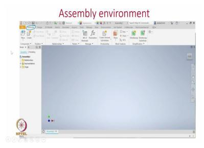
We then enter into the assembly environment. Here is the initial interface of the assembly environment where there are several tabs depending on what is our intent. By default, we start with the assembly tab where we can build an assembly from the components which we will import here from the part models that are already created. So let us get to the software and see how we can start building up assemblies.
