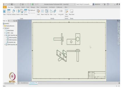
Now let us save it and now open a template for the assembly drawing. So, it is the same as the previous drawings we have looked at. So, we go to these ANSI (mm).idw. So, once we are in this drawing environment, to get the drawings it is the same procedure we used with the part models.
