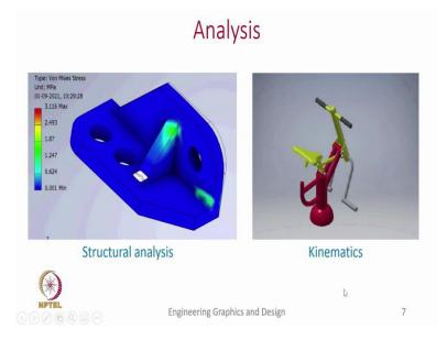
First let us start with analysis. There are many analysis engineers do in an industry or at a workplace. They include structural analysis. Like for example this is a, what I show here is a bracket and once you apply a load it deflects. So, when it deflates, it induces stresses in this object. And as a designer one may need to know whether these stresses are within the allowable limit or not. So, that can be done using the same solid models.
