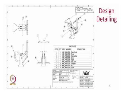
So, let us say we are done with the design process and then one needs to fabricate your device or an instrument. Then you need to approach a third person who fabricates these devices. Usually that third person takes engineering drawing which are more precise. So, for example you can use the same solid model and with a click of a button the CAD software will help you get the design drawings.
