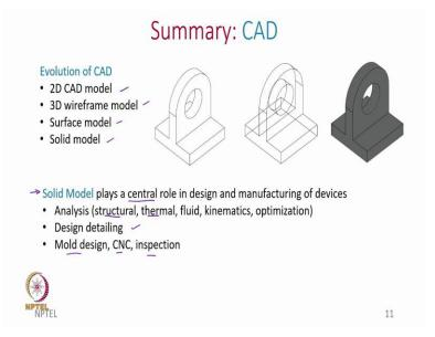
So, let me summarize this lecture. So, we started by looking at the evolution of CAD models where we started with a 2D CAD model, then the 3D wireframe models, surface model and finally the solid model. We said, currently in the industry the solid modelling is a more powerful technique and very commonly used. This solid model is used both in the design and manufacturing. It plays a central role in the design and manufacturing of devices.
