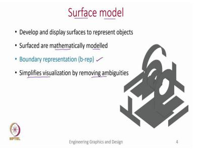
So, over the time there were improvements in the CAD software. Then people started developing these surface models. So, essentially what we do in the surface model is, if you want to show the object you first model all the surfaces of the object, and only show the outer surface of the object, because once you look at the outer surface of the object you will get an idea about how the object looks like in the real world.
