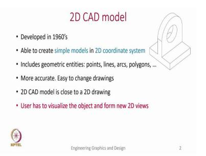
So, let us start with evolution of the CAD software because that helps us understand what are the features of these software and how they have improved over time. So, we will be talking about four different models or the modelling techniques. Initially we will start with this 2D CAD model which were developed in the 1960s. Those were the days of early times of the computers. So, the computational powers were less.
