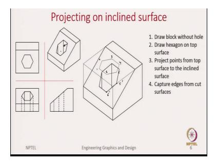
This I will quickly show in the last slide. So again, the same problem so I am not repeating it again. The only difference now I am trying to say is when we draw projection lines, there is one other alternative instead of going to the side view, we can also go into the front view. So, as you can see, we have drawn lines in the top view, then the front view and again the inclined surface and then lastly, we just need to draw vertical lines to project the depth.
