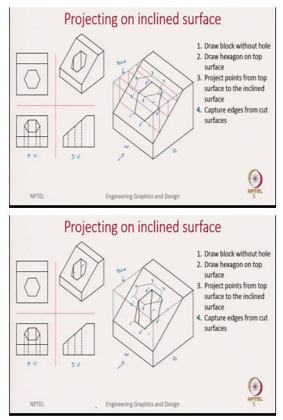
And now let us look at the last example where I want to show how do we project onto an inclined surface. So, these are the orthographic projections are the multi views of an object. As you can see here, I hope you can see that in the top view, you can see a hexagonal cut. But once you look at the front view, and the side view, this hexagonal cut is shown using hidden lines.
