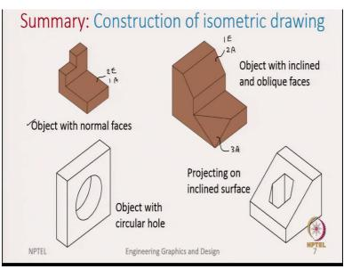
Essentially in summary, what we have seen in this lecture is how do we draw isometric views for an object with normal surfaces, we said a normal surface is one which is parallel to one of the principal planes. So, for example, this surface will look as an edge in two of the principal views but as an area in one of the principal views.
