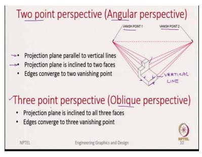
So, now let us look at the two-point perspective, which we also call as the angular perspective. So, here we show the object we are looking at, there are two important points to know. First is the projection plane parallel to the vertical lines. So, for example, if you are looking at this as the vertical line, this as the vertical line, we see that your projection plane is parallel to the vertical line.
