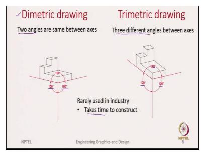
The second is the diametric drawing. Again, the difference is now only two of those angles have are same. So, for example here, this and this are 100 degrees, so both of them are equal, but the third angle is different. So, this is our solid in the dimetric view. So, as you can see, let us say the front face and the side face, both have the same dimension, whereas the height is slightly squeezed.
