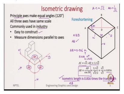
Isometric drawings are the most commonly used drawings, out of all these pictorial drawings. So, what it says is, these are principal axes, which are shown here, they make equal angles. So, as you can look, they are making an angle of 120 degrees with each other. So, you should now realize that these axes in the true sense are perpendicular to each other.
