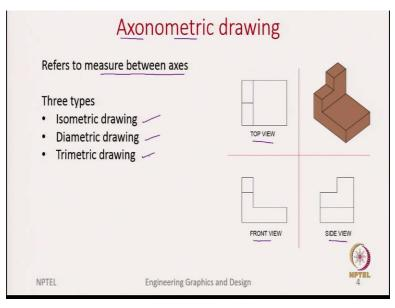
So, now let us start with axonometric drawings. Axon means axes and metric means measures. So, what do they do? They refer to the measurement between the axes. So, we all know we are working with three dimensional objects, so we need to represent it in a three coordinate axes system.
