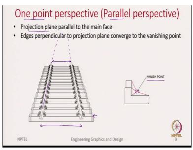
So, here is the one-point perspective also called parallel perspective. So, previously, I was mentioning about you standing in a long corridor, but you can also I think, we have all seen this. At least the picture if not in reality that looking into the tracks, which are railway tracks, which are very long, you have a feeling that these tracks are maybe meeting each other at a far distance.
