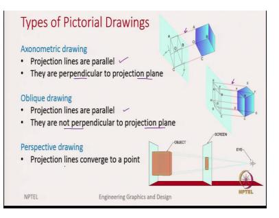
The first category is the axonometric drawings where the projection lines are parallel. So, for example in this picture, we see these red lines are the projection lines and they are all parallel. They are not just parallel, but they also intersect the projection plane at 90 degrees or they are perpendicular to the projection plane.
