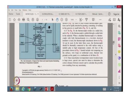
So, it gives us a sketch of what the general arrangement of the system should be. So, there they have said that there is a bar specimen, a meter bar, heater section, guard heater section, and how much distances they should have, and also where we should put the temperature sensors. So, these are all the temperature sensors that are coming here, this one, this one, this one, like that.
