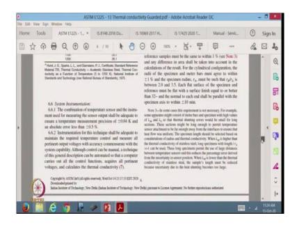
You can have a look at this yourself, but the thing is where is uncertainty coming in. And this is where that it has given some information and it says; the conduction area of the specimen and reference samples must be the same to within 1 percent. The radii of specimen and meter bars must agree to within plus minus 1 percent. Like this there are several things given, and finally in the end it tells us how to compute the errors.
