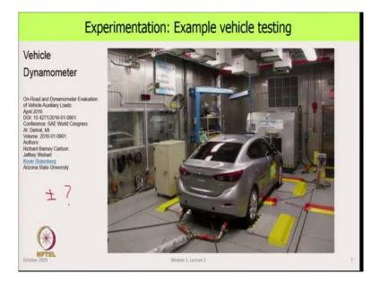
This is the example of a vehicle dynamometer, many students are fascinated by automobiles, but the way the automobile is actually tested is in a facility which you see in this picture this is taken from a website.
