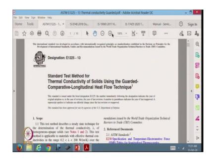
Here is an example which is the standard from ASTM American Society for Testing and Materials, the standard designation is given here at the top and this is E1225, this is ASTM standard E1225 which is the standard test method for thermal conductivity of solids using the guarded comparative-longitudinal heat flow technique.
