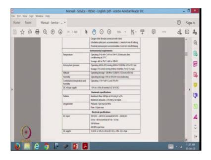
But we will come here, and this table gives us the specifications of the ventilator. This is all weight, dimensions, etcetera, environmental requirements, that is under what conditions it will work. And now pneumatic specifications that its got a turbine whose maximum flow rate is 240 lpm, litres per minute, at 24 centimeters of water column pressure plus minus 1 percent.
