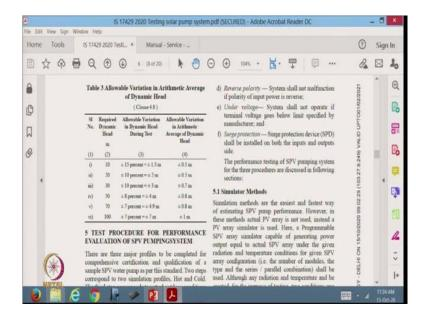
Only then the result that you report for testing the pump that you have will be acceptable and will be meaningful. There is another table here which says allowable variation in arithmetic average of dynamic head that when you are setting up the apparatus how much variation is allowed.
