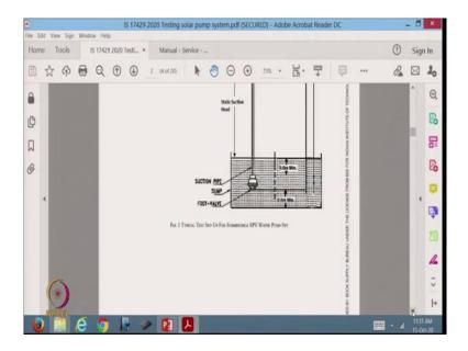
This is the general guidelines for putting it up. There is a sketch which says that right here in the middle we have the pump, the pump controller, solar photovoltaic array, the structure and here it picks up water from a tank below the pump, pumps it through some instrument, there is the flow meter and dumps it into back into the tank.
