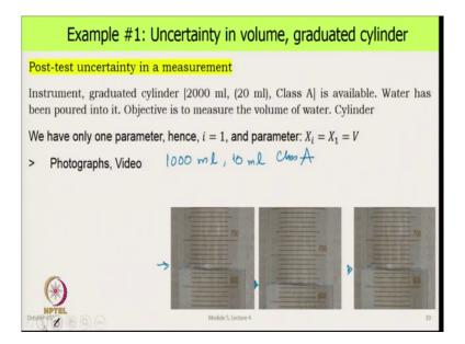
So, we did the experiment in our lab and we use 1000 millilitre measuring cylinder with 10 millilitre markings class A and we have made a video of that and some snaps from that are shown here. So, you can see the water level at this point here, the water level is over here and the water level is somewhere there.
