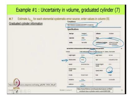
So, this is another example of a graduated cylinder, where it says that it has white round and capacity is 1 litre and tolerance is plus minus 3 millilitres. So, this is what we took in our calculation. Graduations 10 ml, subdivision 10 ml. And it says here Pyrex certified serialized class A cylinders with metric scale. So, question is what is what do they mean by class A cylinders and that is what we looked at this was referring to a standard and that is written over here.
