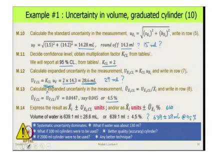
Then, we will do a last sequence of steps which will also take us to table M-3; we will see that in a minute. We calculate the standard uncertainty in the measurement which is square root of this and this which is 14.28, we round it off to 14.3. The question is should I report this as 15? We will come back to it in a minute. Confidence level, we say we will report at 95 percent confidence level, for which our multiplication factor is 2.
