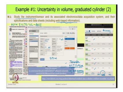
This is from another manufacturer. So, here they have said volumetric cylinder, hard glass, this is a height, then volume tolerance plus minus 5, capacity 1000. So, this is all in millilitres. So, a 1000 millilitre cylinder, their volume tolerance is plus minus 5 millilitres and
