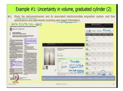
So, now start our step-by-step process to decide what is the uncertainty in the measurement. Our first step is to study this device, the instrument, sensor, electronics and as I mentioned web-based information and even some standards. So, we come across a standard here, which is here ASTEM E1272 dash 02. This is American society for testing and materials.
