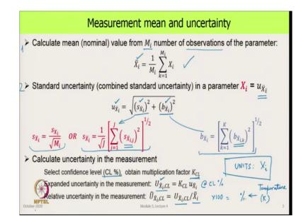
To summarize, the process of estimating measurement, mean and uncertainty takes the following steps. First, we calculate the mean or the nominal value from the various number of
