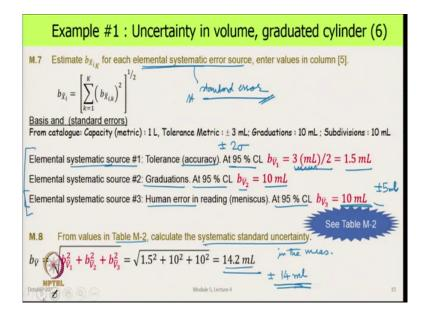
Next, we calculate the elemental systematics errors and since, we have done those three sources. So, we write down here source number 1; systematic error source number 1, tolerance or same as accuracy and here, we go to one of those criteria which is in ISO gum, which says that if the accuracy is reported at 95 percent confidence level, then the standard error associated with that is the value of the accuracy divided by 2 because 95 percent corresponds to plus minus 2 sigma.
