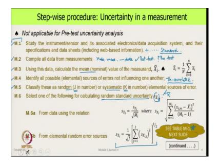
Then, on the same arguments, I have listed here in the step-by-step approach. So, one can follow this procedure, when solving a problem. The step number is indicated over here; M1 denotes measurement first step, study the instrument sensor and its associated electronics or data acquisition system and their specifications and data sheets including web-based information and anything else that you can learn about that measurement.
