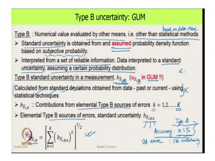
Type B uncertainty is somewhat different, X i in Type B numerical value of the uncertainty is evaluated by what is written as other means. That means, other than statistical methods based on recorded data and data we mean measurements data.
