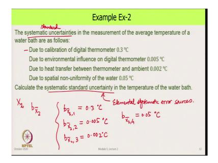
Now, we come to the next example it says the systematic uncertainties in the measurement of the average temperature of a water bath are as follows, due to calibration of digital thermometer 0.3 degree Celsius due to environmental influence on digital thermometer 0.005 degree Celsius, due to heat transfer between thermometer and ambient 0.002 degree Celsius.
