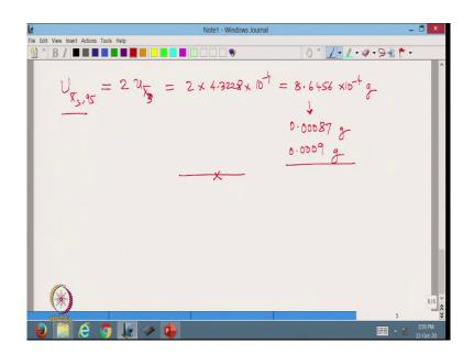
And then in the next step we have to calculate u X 3 bar at 95 percent confidence level this is 2 u X 3 bar which is 2 times that number we got 4.3228 into 10 to the power minus 4 which is 8.6456 into 10 to the power minus 4 grams which we round off to 8.2 0.00086 or 0.00087 we can say or even 0.0009 grams either of those would be ok.
