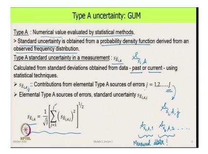
Now, according to this guide sources of error are classified as Type A and Type B. Type A errors are causes of errors result in an uncertainty which is evaluated by statistical methods.
