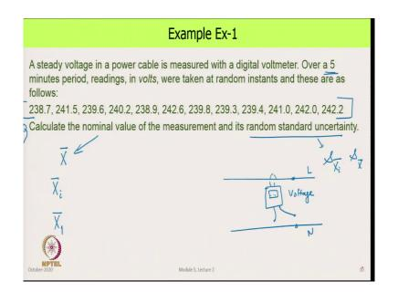
Here is the first one the application is that there is a electric cable around that we have put an instrument which is a voltmeter or a multi meter and we are reading the voltage based on the way it picks it up. This thing the current and there will be another 2 links which are connected between the supply lines this is say the live and neutral or Earth and we are getting the voltage between these two.
