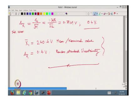
So, we keep all those twelve readings and go ahead and now our job is to calculate X 1 X bar which is the standard error or standard deviation of the mean which is s X 1 1 which is the sample standard deviation divided by the sample size which is 1.386 divided by square root of 12 and this turns out to be 0.3949 volts which we round off to 0.4 volts.
