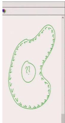
Figure 10: Shear stress distribution along the periphery of the cross-section of a beam when the lateral surface of the beam is traction free
