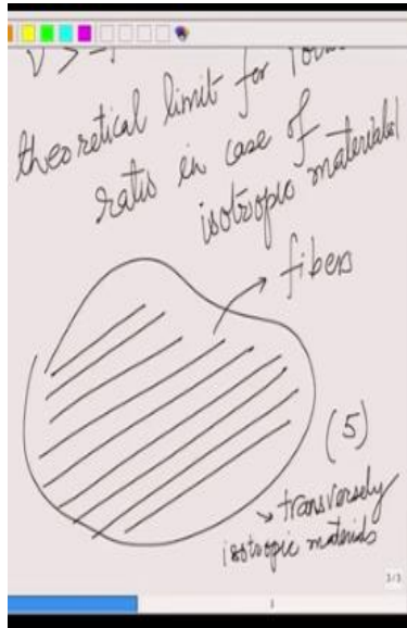
Figure 7: An initially isotropic material is engraved with fibers
