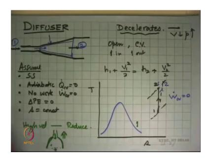
And the opposite of the nozzle is what is called a diffuser. So, generally look at what is the diffuser now. So, this is a thing which decelerates the fluids that means, in the direction of flow, the velocity goes down and pressure goes up. So, what is happening here is that we have a flow coming in, and then there is the area opening up, and the flow goes out over there.
