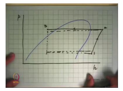
And then the diagram is look very simple will actually start looking a little more complicated, I will just make one diagram at the illustration, and this is on the ph diagram. So, this is the dome, and the ideal cycle says this is the compressor outlet, this is the compression process, this is inlet, this is outlet.
