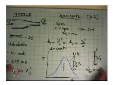
So, let us start with the nozzle. So, this is a device, which accelerates a fluid in the process the pressure drops. And a typical sketch of this would look like this in which the working substance enters here, and exit over there. And we make this as a system saying that the system boundary is everything that is inside this nozzle, and in that we apply various laws.
