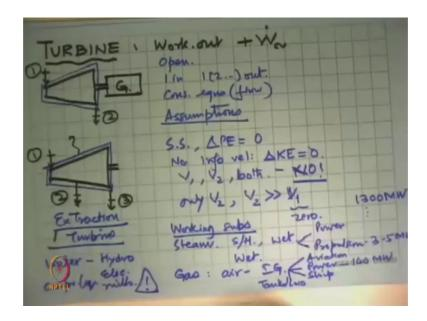
And the next thing we look at is a turbine. These turbine, steam turbines are used largely for power generation and also in the case of ships and submarines for propo the (Refer Time: 00:41) nuclear submarine or a nuclear aircraft carrier which have the nuclear reactor which produces steam and steam runs a steam turbine gas turbines also stationary like power generation gas turbines are also (Refer Time: 01:05).
