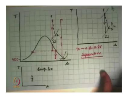
Now, you see what it looks like on property diagram. It is a T s diagram it is a looking at steam turbines, we have to show the dome, and in this case the mentioned in the what you like to do is avoid a two phase mixture inside those machine like the turbine.
