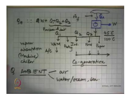
There are other ways by which you can maximize the utilization of your Q H. So, I will take a few minutes to go into this. And what we will does, it says that look I when use the cycle and when I reject the energy, I get some work out some (Refer Time: 39:50) Q H, which is by burning of the fuel. But, now I would be at slightly different thing, I would not explained it, all the way down to 45 degree Celsius, I would not cool it down, but I will keep it at say 100 degrees Celsius.
