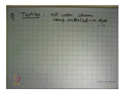
There is a question here, what are the applications of thermodynamics in textile field. One of the big applications of thermodynamics in textile field is that in many textile operations, we need either hot water or steam or a temperature controlled system for certain things to take place; for example, for say dye or for processing of yarn things like that.
