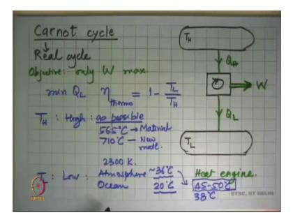
And now we go back and ask a question that has come up, and let us take some time on that. And the question is that why is Q 2, which is lost to the low temperature reservoir in a heat engine operation cannot be recovered completely or partially. So, here is what the question means, you have a high temperature reservoir, a low temperature reservoir, this took heat from here Q H. And dumped some heat into the low temperature reservoir Q L, and in the process gave us work.
