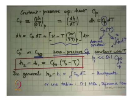
So, the next thing we have to do is we define two properties. The first is constant pressure specific heat we denote this by c p and its defined as dh by dt at constant pressure, ok. So, that is what we have and we can also write this we want as dh is equal to c p dt for constant pressure process.
