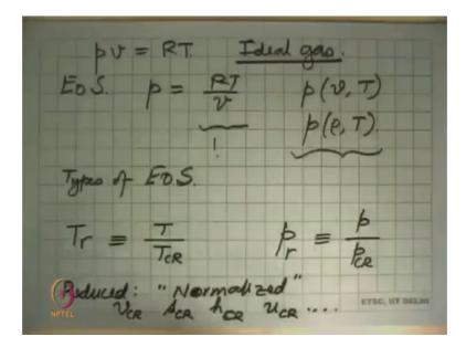
So, familiar with p v equal to RT this present apply to the vapor states and this applies when we do an ideal gas and this is the simplest form of the equation of state is called let us say EOS where we have p is equal to RT upon v.
