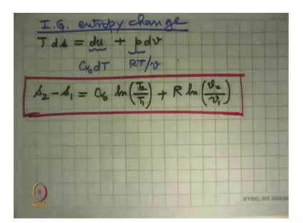
S is equal to du plus p dv and here we make the substitutions there before du. We now know is C v 0 dT and p is r t upon v. The ideal gas equations state ideal this is ideal gas entropy change and like before we do that simple calculation simplification y integration and you get s 2 minus s 1 is C v 0 ln t 2 by t 1 plus r ln v 2 by v 1 and that is the 2nd equation that we have been looking for.
