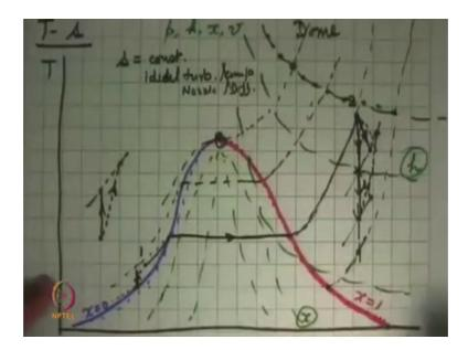
So that was the p-h diagram, we now go to the next type of a diagram which is again very popular in use is temperature entropy diagram. On the y axis is temperature, and on the x axis is specific entropy. And again making this plot we have to be we have to of the same caution that we had with the p-h plot. Once you have set specific entropy at a particular point to 0 specific entropy also gets set to 0.
