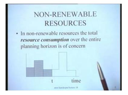
Here our concern is primarily with the total area or the total consumption. Consumption is nothing but the area under the resource usage profile. On the other hand if we look at renewable resources, here the concern is with the total resource usage at each point of time.
