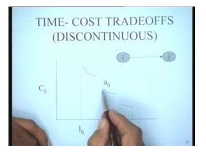
The next stage of technology would be to start using a tractor. When you use a tractor your duration is going to be much smaller and there also depending upon the usage of the tractor you could be having a range of durations. This kind of typical discontinuous time-cost trade off can be utilized when you have different choices, multiple choices as you have in this case. It's like changing of technology from one to the second to the third and you have this kind of change over.
