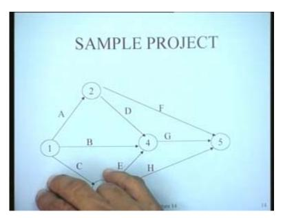
Let us now give the data for this problem. Before giving the data we just like to specify how the cost slope is computed. For linear time-cost tradeoffs you have the activity cost and the activity time on this side. Cost slope for any activity is nothing but the crash cost. It's actually this upon this. It's the crash cost minus the normal cost which is this distance divided by the normal duration minus the crash duration. It's as simple as that. (Refer Slide Time: 21:03)
