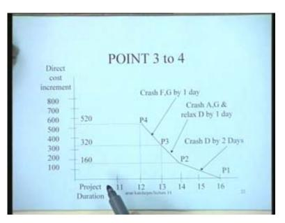
The total cost goes up from 320 to 520 corresponding to point 4. We have moved from point 3 to point 4 and we have come to project duration of 12 from 13 when we were at point 3. This is the manner in which we have moved.
