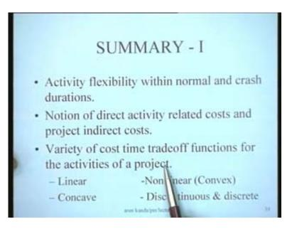
You might talk of linear, non-linear convex or concave or discontinuous and discrete time-cost trade off functions to represent different situations.
