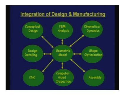
This is one of the slides which we have seen is when you have applications specific package or when you have a integrated environment, when you have to move from one package to another, the geometric model become central and the data exchange becomes a necessity.
