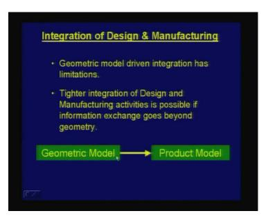
So if I want a tighter integration of design and manufacturing, information exchange should go beyond geometry. So I move from geometric model to what is called as a product model. In a product model geometry is a subset but it includes many other information's which are usually needed for taking certain decisions.
