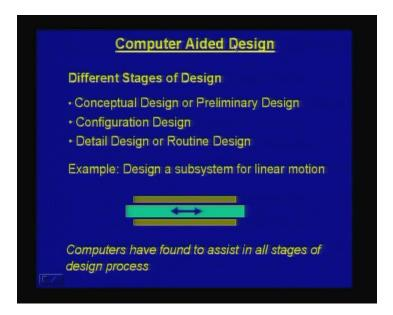
Now design is, the process of design is something which is difficult to layout or to algorithmise but it is believed that computer aided design or in general a design consist of a, it can be classified into three primary stages what is called as a first stage is a conceptual design or a preliminary design.
