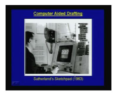
What you see here is basically one of the first computer aided drafting system which was designed in 1963. So this is called as a sketch pad which is basically, the system called sketch pad was designed by Sutherland's at MIT and this is considered to be a beginning of a computer aided design. So we can say that computer aided design is approximately about 40 years old which started with computer aided drafting and then computers where being used in other stages or other aspects of design tool.
